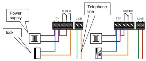
Wiring of standard and magnetic (inverse) lock
